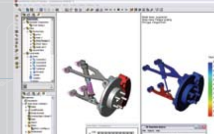
Perform Motion analysis on assemblies with COSMOSMotion, then transfer Motion loads to COSMOSWorks on parts. Predict fatigue life/damage of assemblies with components having different material properties and failure characteristics [S-N curves]
