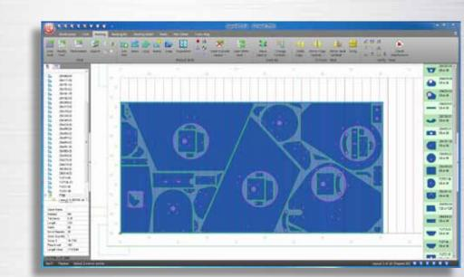
Remnant nesting: Laying out parts on a previously cut "left-over" piece of raw material.
