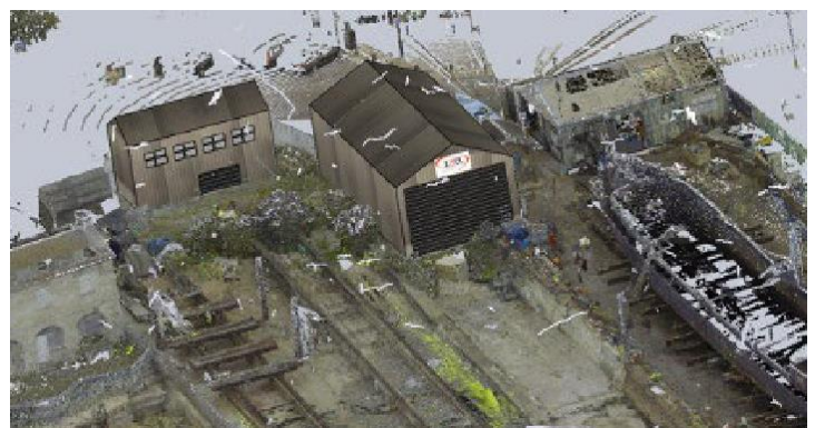
A close up of EAPL's proposed buildings in situ alongside as-built data from the point cloud.
