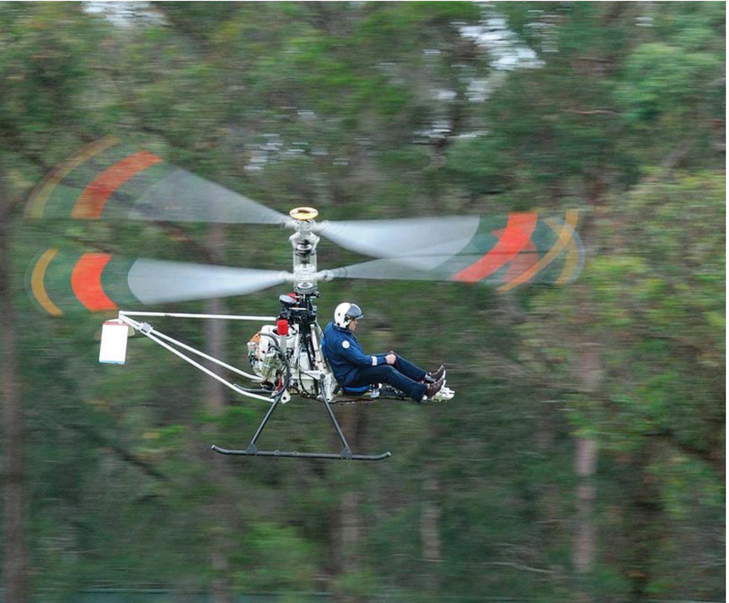
Coax Helicopters leverages SOLIDWORKS Premium design and SOLIDWORKS Composer technical communication software to commercialize coaxial rotor helicopter technology—previously used only by the military—for use in manned and unmanned applications.
