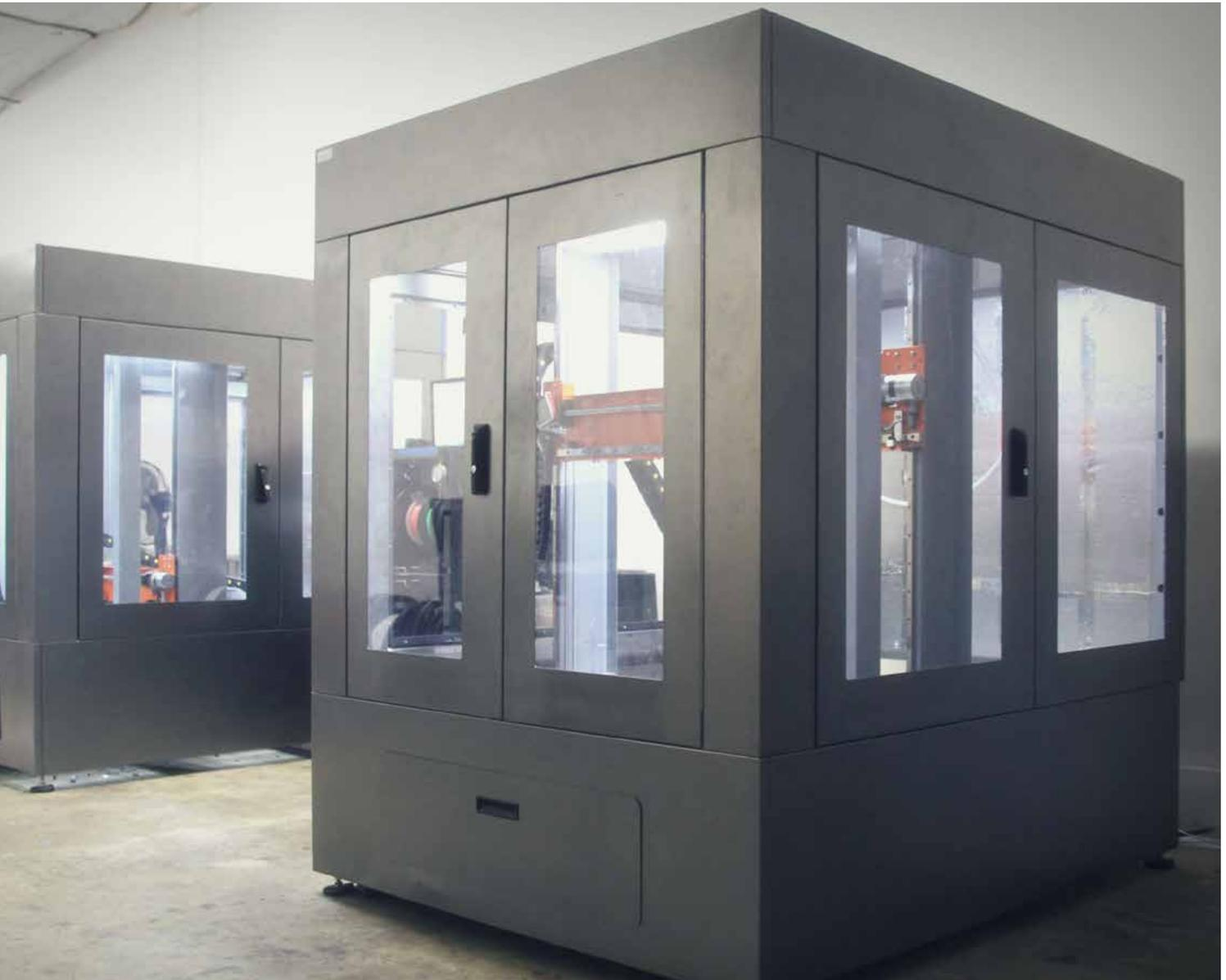
Cosine Additive leveraged SOLIDWORKS design tools to accelerate development of the Agile Manufacturing 1 (AM1), the first large-format 3D printer designed for fabricating highly functional components in a large build envelope. AM1 extends the usefulness of 3D printing technology beyond rapid prototyping, and into actual manufacturing of sizable parts like kayaks and aircraft wings.
