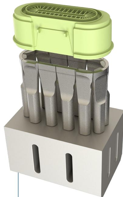
TELSONIC’s ultrasonic tools weld pieces together by using vibration oscillations to generate intramolecular frictional heat, and the company’s engineers rely on SOLIDWORKS Simulation Professional software to quickly run modal analyses and predict frequency modes with a high degree of accuracy to support this process.
