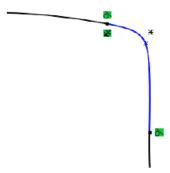
Reference points are displayed for the curve's shoulder and top vertex. Tangent relations are created between the curve and the original sketches.
