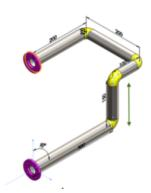
If one end of the pipe route is fixed, then vertical segments of the route are shortened or lengthened to accommodate the sloped pipe segment. If the other end of the pipe
