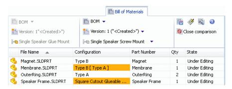
The left section shows the BOM, version, and configuration that are the source of the comparison. The middle section lets you choose the BOM, version, and configuration to compare. In the commands section on the right, the **Comparison** button becomes a **Close comparison** button.
