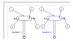
In this example, the block on the right is added to the drawing view, rather than replacing the drawing view on the left.
