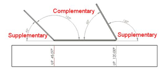
In a drawing with a flat pattern view of a sheet metal part, select the drawing view. Set options in the Drawing View PropertyManager under **Bend Notes**.
