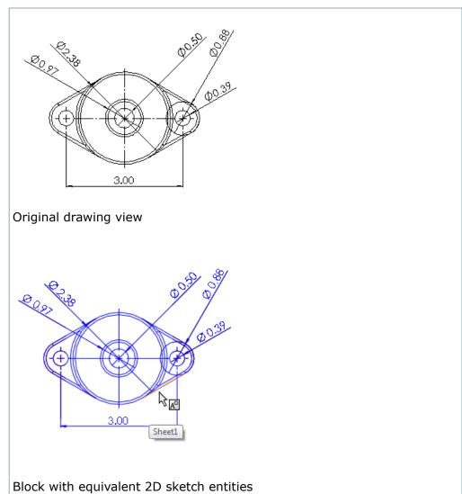
**Insert as** Creates a separate block comprised of equivalent 2D sketch entities that you can place anywhere in the drawing.
