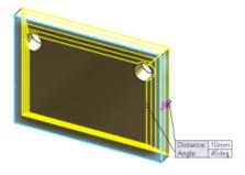
b) Create a new global variable in **Distance** ♦ by typing =chamfer and click ✔ in the input field.
