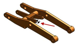
The COM point can be suppressed and unsuppressed for configurations.
