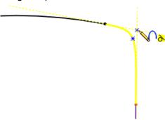
You can snap to the intersection of both inference lines to choose the top vertex of the conic curve.
