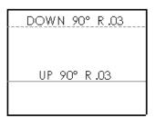
To access or change the edge types, click **Tools** > **Options**. On the Document Properties tab, click **Line Font** and under **Type of edge**, click **Bend Up, Flat Pattern** or **Bend Down, Flat Pattern**.
