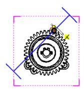
6. Move the pointer to the location as shown and click to set the angle of the cutting line.
