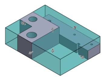
The Costing tool computes the contribution of the volume features to the total cost of machining the part.
