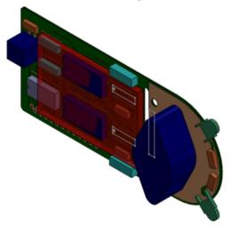
When the SolidWorks model appears, the traces, layers, vias, pads, holes, and filled areas are included in the SolidWorks FeatureManager design tree.
