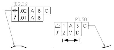
Previously, bent leaders attached to the dimension text. For legacy purposes, existing dimensions remain as they were originally placed.
