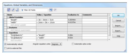
For example, you can create a global variable Length and define it by the equation: =100in + 3mm + 5cm. The equation includes values with three different units of measurement. If the unit of measurement of the document is inches, then Length evaluates to 102.087in. If you change the unit of measurement of the document to millimeters, then Length automatically evaluates to the value of 2593mm. You do not need to edit the equation, or be concerned that the size of the part will change.
