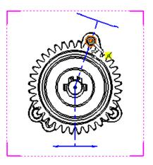
7. Move the initial side of the second cutting line to the location as shown and click.
