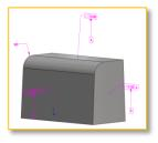
Used to fully constrain a model with dimensions, datums and tolerances. This makes drawing creation much quicker as the dimensioning scheme is already done. Is also a prerequisite for the **TolAnalyst** stack up add-in.
